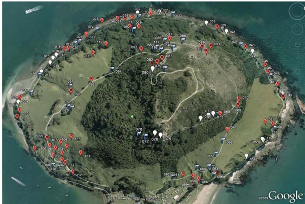
Map showing all of the slips that were identified after the January storm event.
